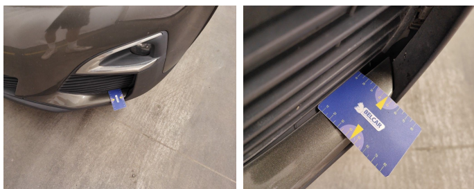
Bumper Front / Trim Left / Replace-bad position
