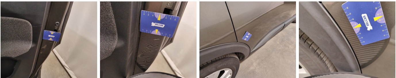
Door Rear Right // Repair & Painting-scratch + dent
