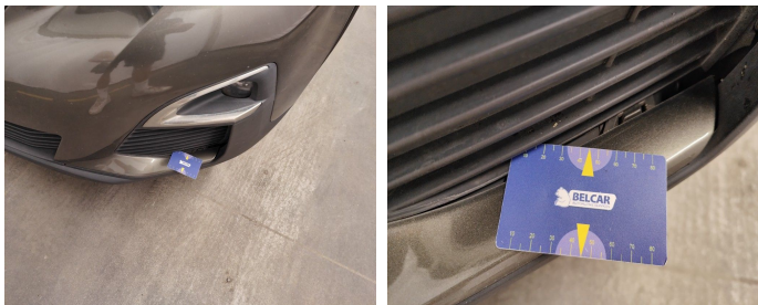
Bumper Front / Grid Left / Replace-bad position
