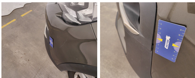
Bumper Front / Trim Left / Replace-bad position
