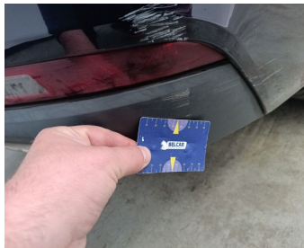
Bumper Rear / Lower Cover Not Painted / Replace-scratch
