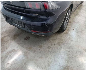
Bumper Rear / Lower Cover Not Painted / Replace-scratch
