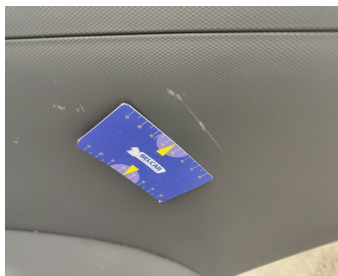
Interior / Side Cover rear Seat / Replace-scratch
