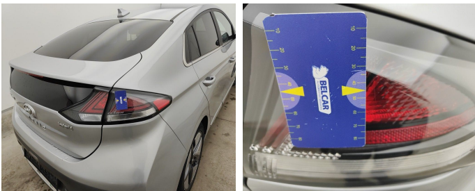
Light / Rear Right / Replace-scratch
