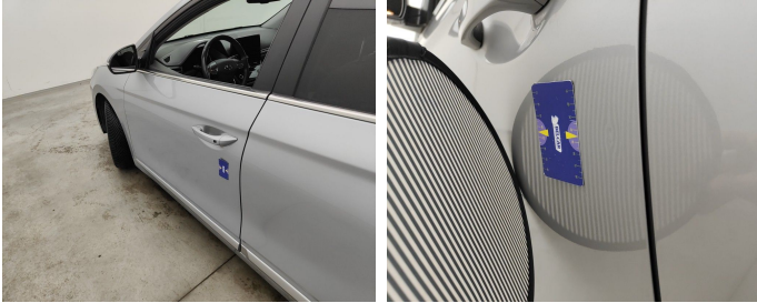
Door Front Left // Smart Repair Small-dent
