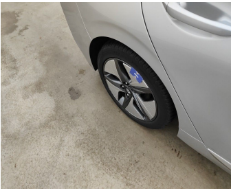
Tyre Rear Right // Replace-worn
