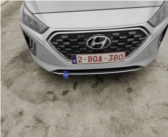
Bumper Front / Spoiler / Replace-stone chipping
