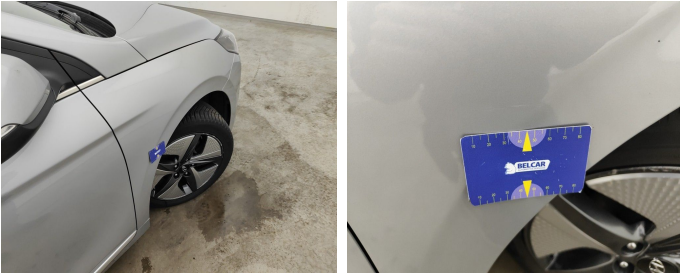
Wing Front right // Polish-scratch
