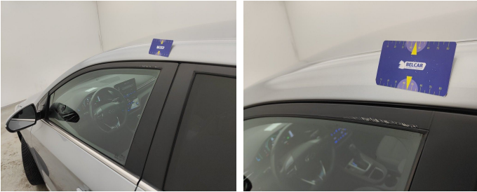
Door Front Left / Trim / Replace-Chemical reaction
