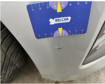
Bumper Front // Painting-stone chipping
