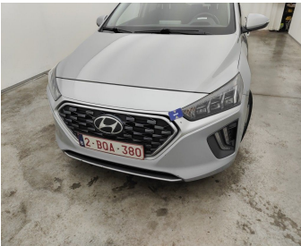
Bumper Front / Trim Right / Replace-stone chipping
