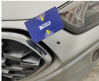
Bumper Front / Trim Right / Replace-stone chipping
