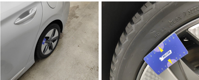
Tyre Rear Left // Replace-tear
