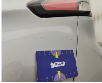
Wing Rear Left // Repair & Painting-scratch + dent
