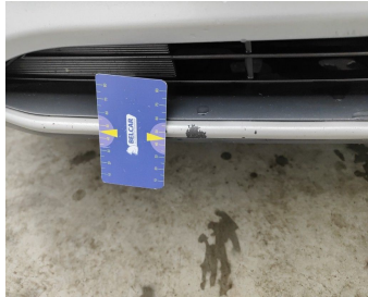
Bumper Front / Spoiler / Replace-stone chipping
