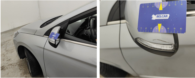
Side View Mirror Left // Painting-scratch
