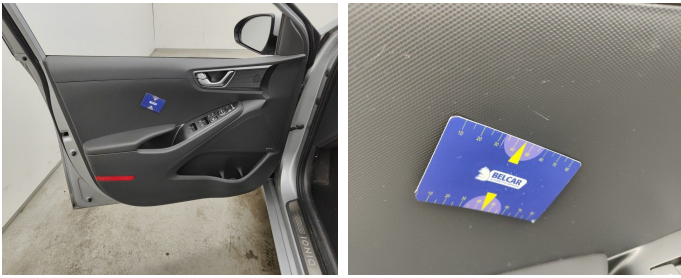
Front Left Door Interior Coating // Replace Completely-scratch
