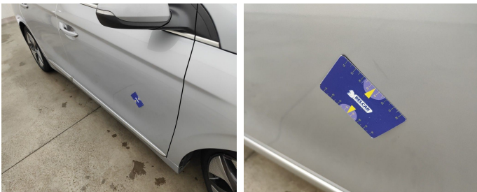
Door Front Right // Polish-scratch
