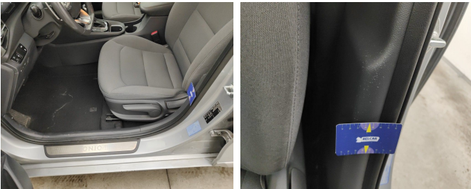
Interior / A Pillar Lower Cover / Replace-scratch
