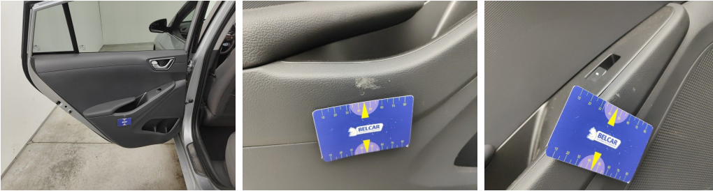
Rear Left Door Interior Coating // Replace Completely-scratch
