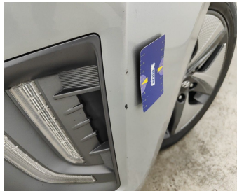
Bumper Front / Trim Right / Replace-stone chipping
