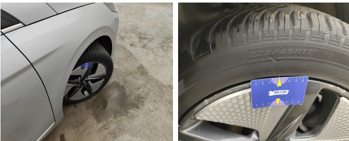
Tyre Front Right // Replace-tear
