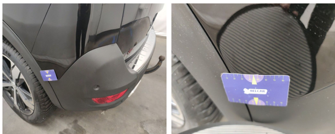
Bumper Rear // Painting-bad repair
