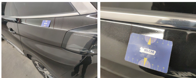
Wing Rear Left // Painting-bad repair
