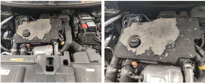
Front Bonnet / Insulation / Replace-cracked
