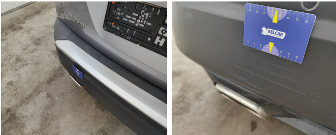
Bumper Rear / Lower Cover Not Painted / Replace-scratch
