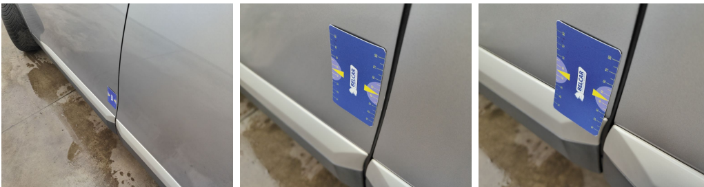
Door Front Left // Smart Repair Small-scratch
