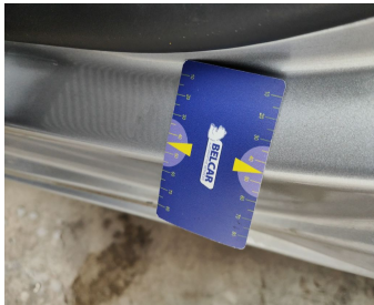
Rocker Panel Left // Smart Repair Medium-scratch + dent
