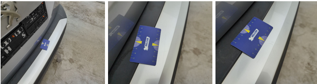
Bumper Rear / Trim Center / Replace-scratch
