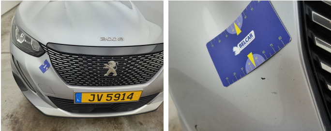
Bumper Front // Painting-stone chipping
