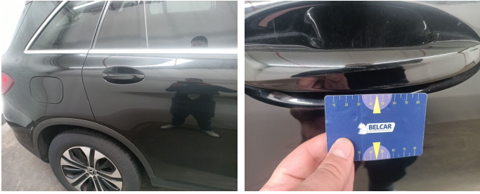
Door Rear Right // Smart Repair Medium-scratch
