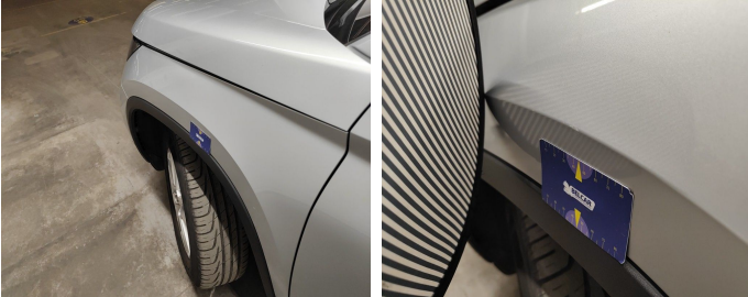
Wing Front Left // Repair & Painting-scratch + dent
