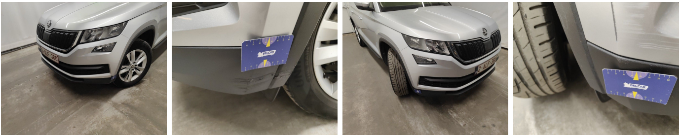
Bumper Front / Lower Cover Not Painted / Replace-scratch
