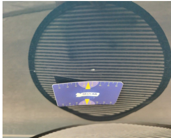
Door Front Left // Repair & Painting-dent
