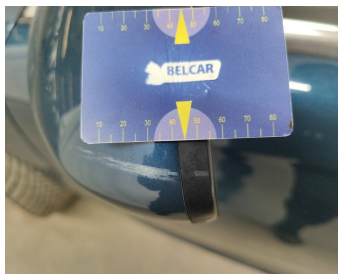
Side View Mirror Left // Painting-scratch
