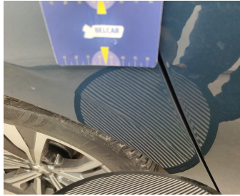
Wing Rear Right // Painting-bad repair
