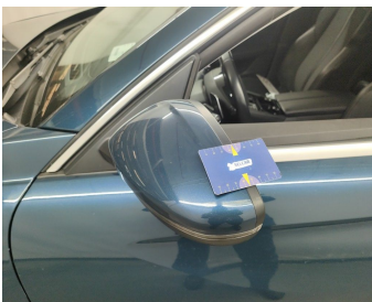
Side View Mirror Left // Painting-scratch
