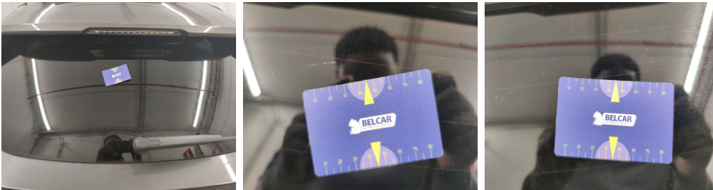
Rear Bonnet / Rear Window / Replace-scratch
