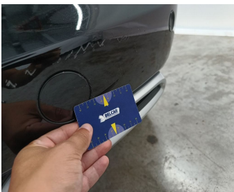
Bumper Rear // Painting-scratch
