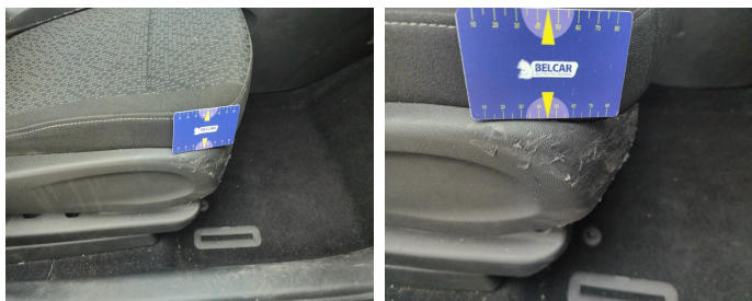
Seat Front Right // Repair-scratch
