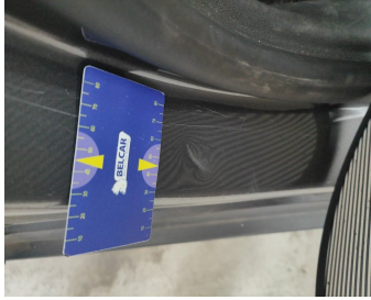
Rocker Panel Right // Repair & Painting-scratch + dent
