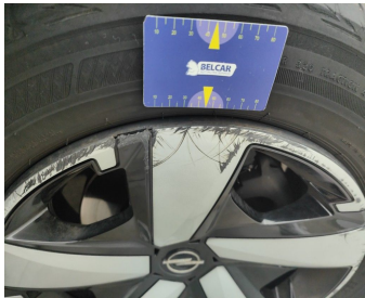
Wheel Front Right / Wheel Cover / Replace-scratch
