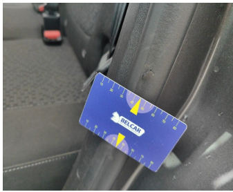
Door Rear Left // Smart Repair Medium-tear
