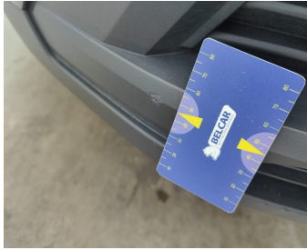
Bumper Front / Lower Cover Not Painted / Replace-scratch
