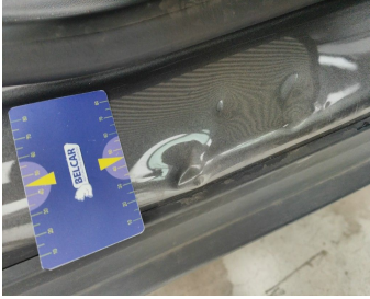
Rocker Panel Right // Repair & Painting-scratch + dent
