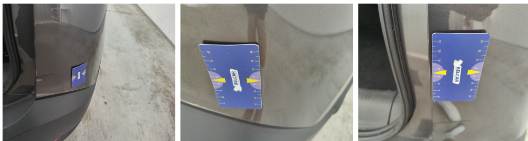
Bumper Rear // Smart Repair Medium-scratch
