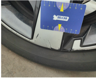
Wheel Front Left / Wheel Cover / Replace-scratch
