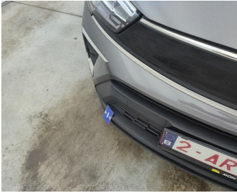
Bumper Front / Lower Cover Not Painted / Replace-scratch
