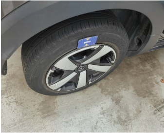
Wheel Rear Right / Wheel Cover / Replace-scratch
