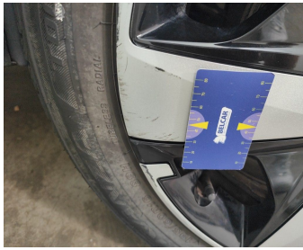
Wheel Rear Left / Wheel Cover / Replace-scratch
