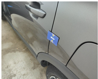
Wing Rear Right // Smart Repair Small-dent
