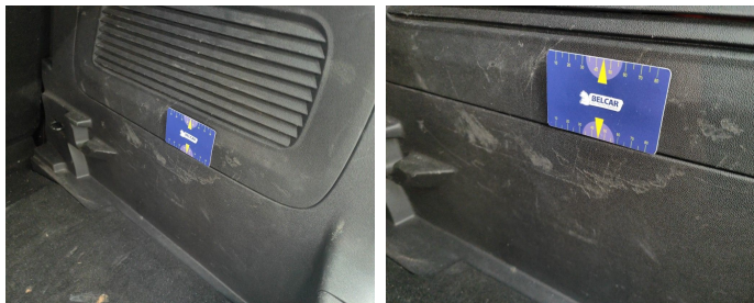
Trunk Compartment / Side Cover Right / Replace-scratch
