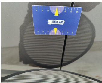
Wing Rear Right // Smart Repair Small-dent
