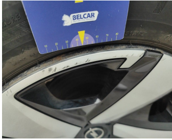
Wheel Rear Right / Wheel Cover / Replace-scratch
