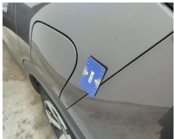
Wing Rear Left // Smart Repair Small-scratch + dent
