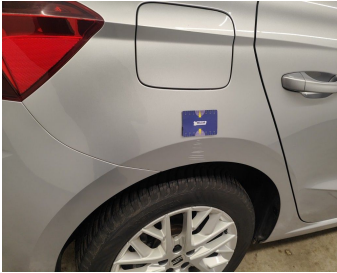
Wing Rear Right // Painting-scratch
