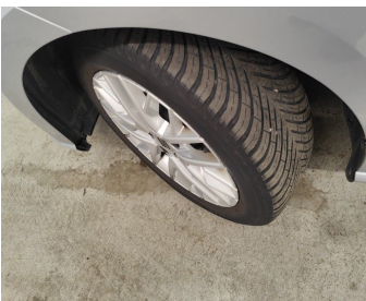
Tyre Front Left // Replace-worn
