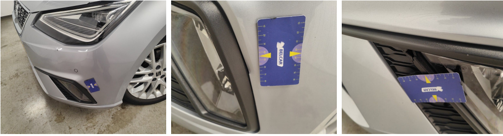
Bumper Front / Trim Left / Replace-cracked
