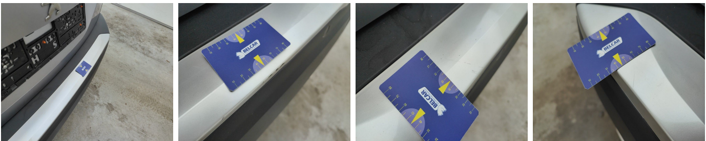
Bumper Rear / Trim Center / Replace-scratch
