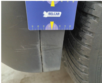
Wing Rear Right / Trim / Replace-scratch
