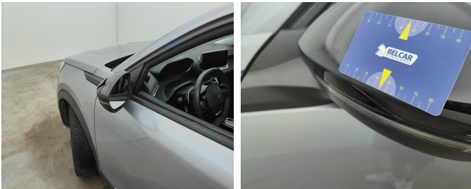
Side View Mirror Left // Painting-scratch
