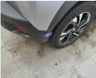
Wing Rear Right / Trim / Replace-scratch
