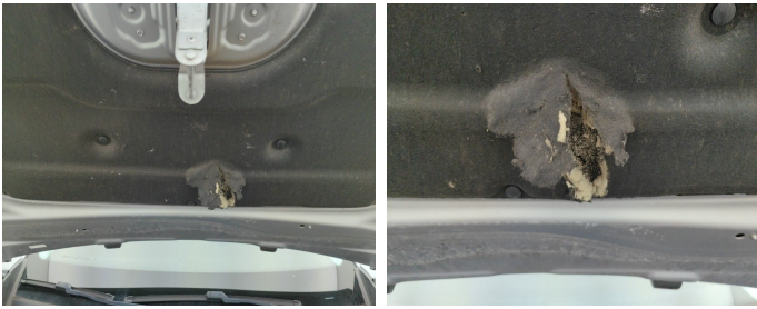
Front Bonnet / Insulation / Replace-tear
