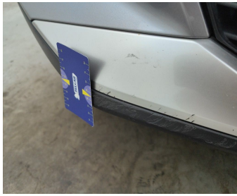
Bumper Front / Lower Cover Not Painted / Replace-scratch
