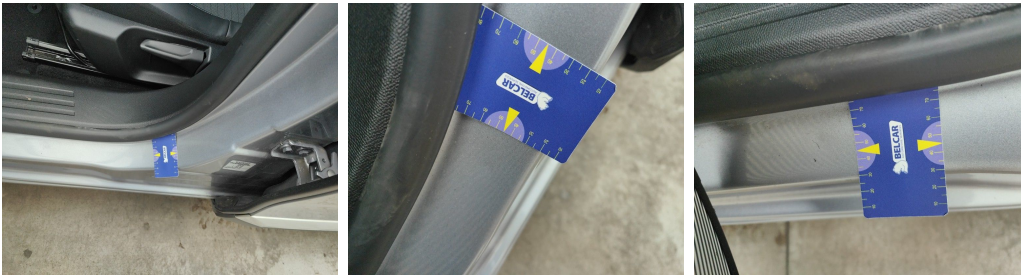
Rocker Panel Left // Smart Repair Medium-dent
