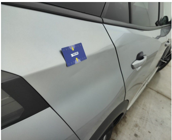
Wing Rear Right // Repair & Painting-scratch + dent
