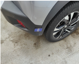
Bumper Rear / Lower Cover Not Painted / Replace-scratch
