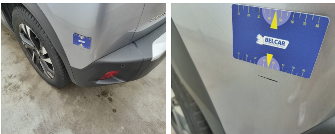
Bumper Rear / Trim Center / Replace-scratch
