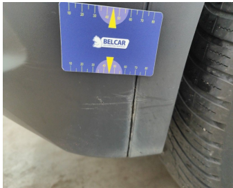
Bumper Rear / Lower Cover Not Painted / Replace-scratch
