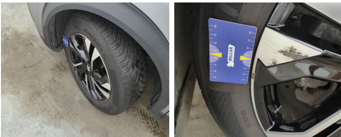
Wheel Two Tone Front Left // Repair-scratch
