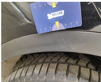
Wing Rear Right / Trim / Replace-scratch
