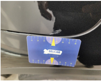
Damage within Renta-norm-scratch
