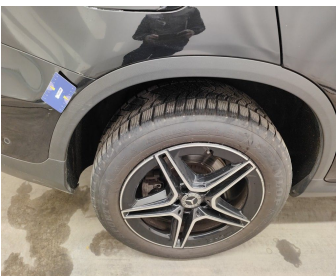
Wing Rear Right / Trim / Replace-scratch
