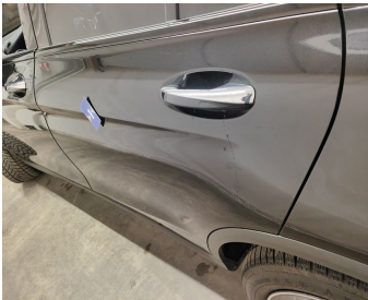
Door Rear Left // Smart Repair Small-dent
