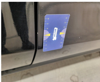
Door Front Right // Smart Repair Medium-scratch
