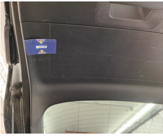
Trunk Lid Interior Coating / Complete Panel / Replace-scratch
