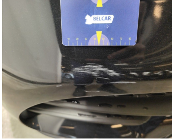
Bumper Front // Smart Repair Medium-scratch
