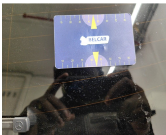
Rear Bonnet / Rear Window / Replace-scratch
