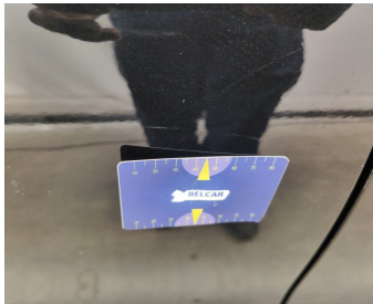
Bumper Front // Smart Repair Medium-scratch
