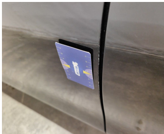
Door Front Left // Smart Repair Medium-scratch
