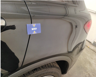
Wing Rear Left // Smart Repair Small-dent
