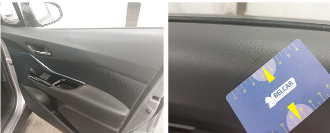
Front Right Door Interior Coating // Replace Completely-scratch
