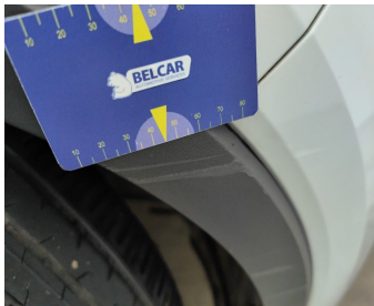
Wing Front right / Trim / Replace-scratch
