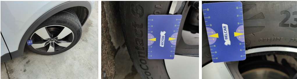
Tyre Front Right // Replace-tear
