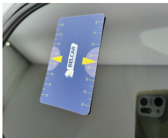
Door Rear Right / Window / Replace-scratch
