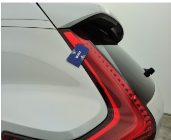
Light / Rear left / Replace-scratch
