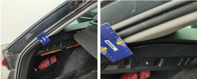
Trunk Compartment / Side Cover Left / Replace-scratch
