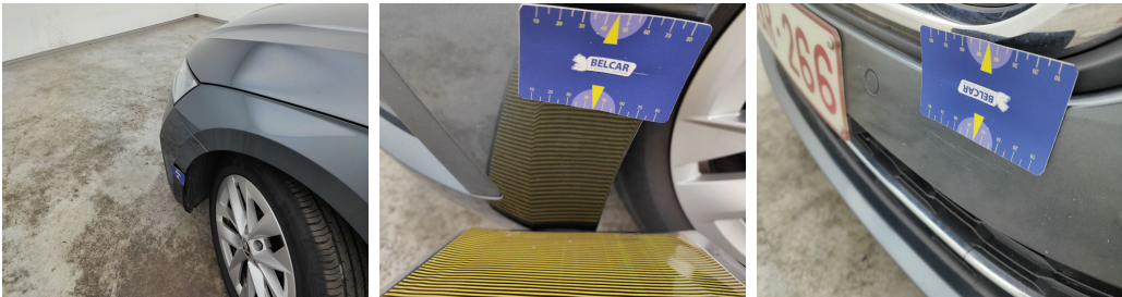
Bumper Front // Repair & Painting-dent
