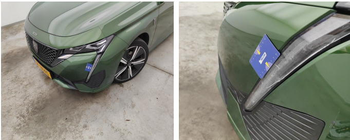
Headlight / Front left / Replace-cracked
