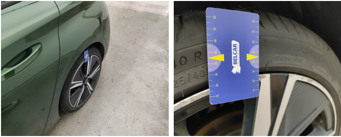
Tyre Rear Left // Replace-tear
