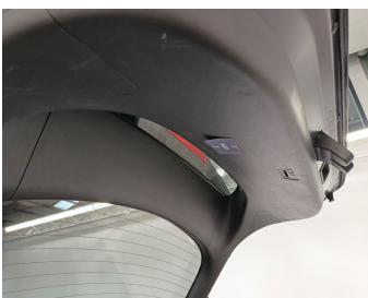
Trunk Compartment / Side Cover Left / Replace-scratch
