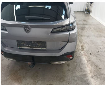
Bumper Rear / Spoiler / Replace-cracked
