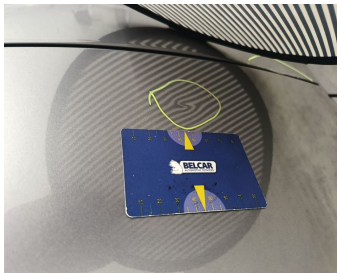
Door Rear Right // Smart Repair Small-scratch + dent
