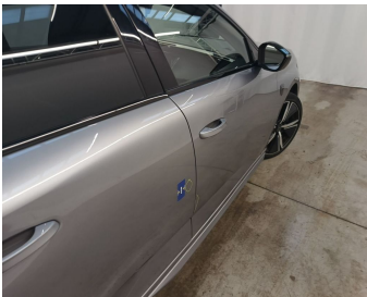
Door Rear Right // Smart Repair Small-scratch + dent
