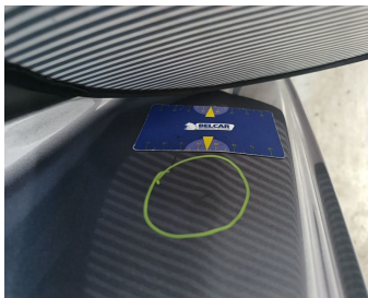
Rocker Panel Right // Smart Repair Medium-scratch + dent
