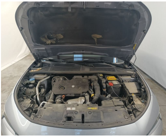
Front Bonnet / Insulation / Replace-tear
