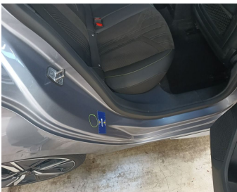
Rocker Panel Right // Smart Repair Medium-scratch + dent
