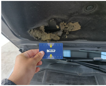
Front Bonnet / Insulation / Replace-tear
