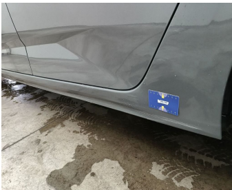
Rocker Panel Left // Repair & Painting-scratch + dent
