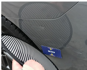
Rocker Panel Left // Repair & Painting-scratch + dent
