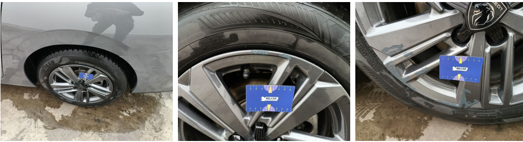
Wheel Alloy Rear Left // Repair-bad repair
