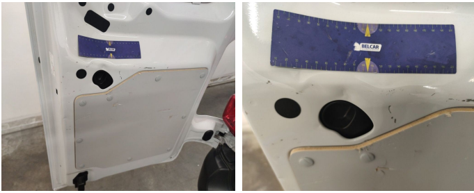
Rear Loading Door Left // Repair & Painting-scratch + dent
