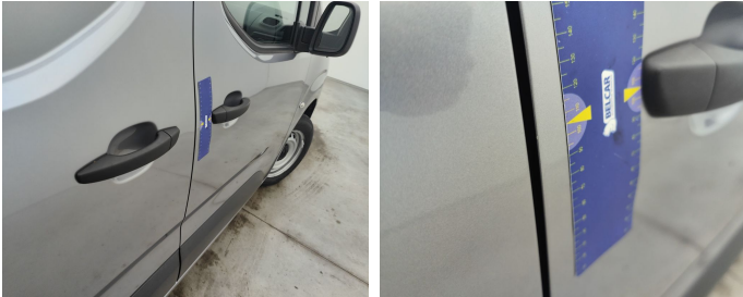
Door Front Right // Smart Repair Small-dent
