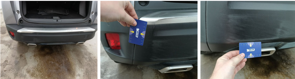
Bumper Rear / Lower Cover Not Painted / Replace-scratch
