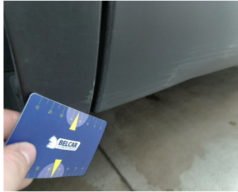
Wing Rear Right / Trim / Replace-scratch
