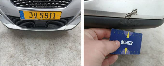
Bumper Front / Lower Cover Not Painted / Replace-scratch
