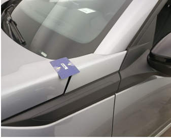
Wing Front Left // Painting-scratch
