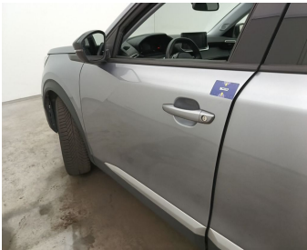
Door Front Left // Repair & Painting-scratch + dent
