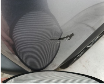
Bumper Rear // Replace & Painting-scratch + dent
