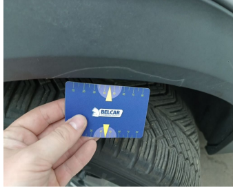
Wing Front Left / Trim / Replace-scratch
