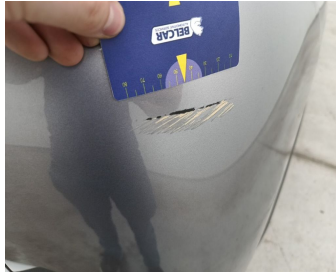
Wing Front right / Trim / Replace-scratch
