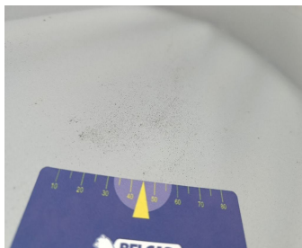
Rear Bonnet // Polish-Chemical reaction
