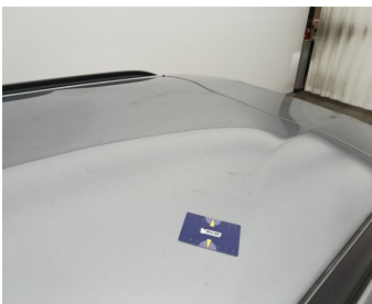
Roof // Polish-Chemical reaction
