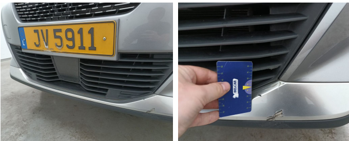
Bumper Front / Grid Central / Replace-scratch
