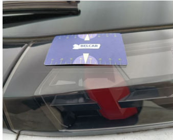
Light / Rear Right On Rear Bonnet / Replace-scratch
