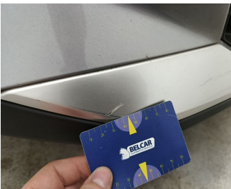
Bumper Front / Spoiler / Replace-scratch + dent
