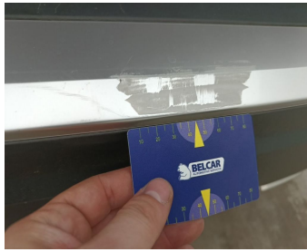
Towing Cover Rear // Replace-scratch
