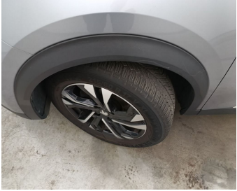
Wing Front Left / Trim / Replace-scratch
