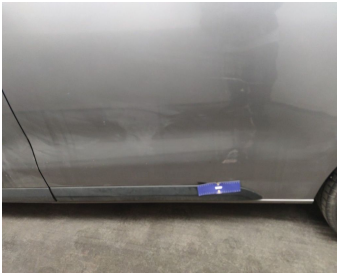
Rear Loading Door Left // Painting-scratch
