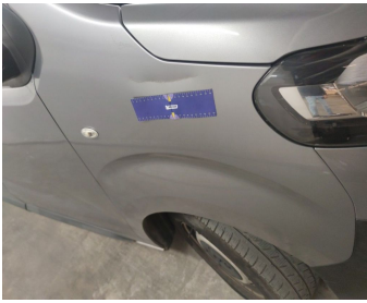
Wing Front right // Repair & Painting-scratch + dent
