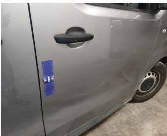
Door Front Right // Painting-scratch
