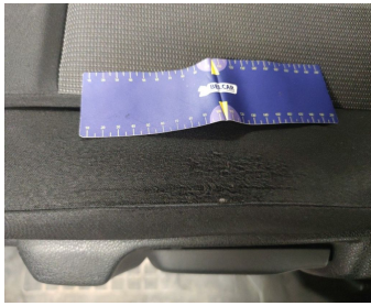
Seat Front Left / Bottom Coating / Replace-worn
