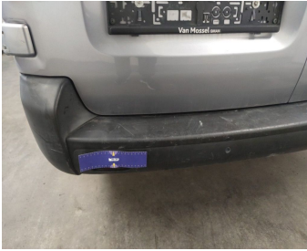
Bumper Rear / Lower Cover Not Painted / Replace-cracked
