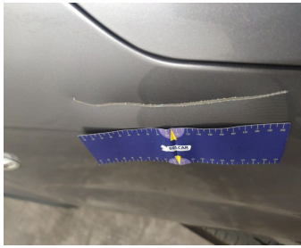
Wing Front right // Repair & Painting-scratch + dent
