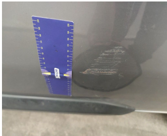
Wing Rear Left // Repair & Painting-scratch + dent
