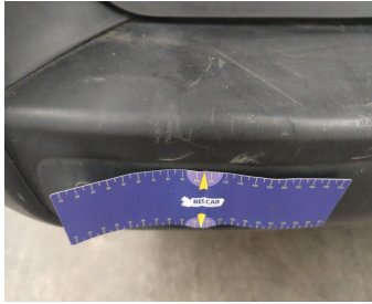
Bumper Rear / Lower Cover Not Painted / Replace-cracked
