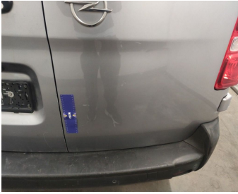
Rear Loading Door Right // Painting-scratch
