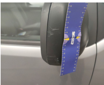
Side View Mirror Right // Replace Not Painted-scratch
