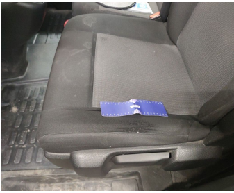
Seat Front Left / Bottom Coating / Replace-worn
