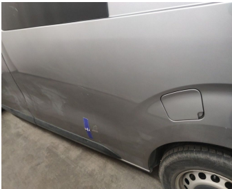
Wing Rear Left // Repair & Painting-scratch + dent
