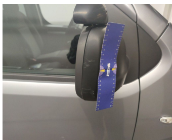
Side View Mirror Right // Replace Not Painted-scratch
