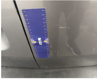
Rear Loading Door Right // Painting-scratch
