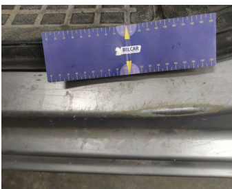
Rocker Panel Left // Smart Repair Medium-scratch
