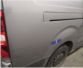
Wing Rear Right // Painting-scratch
