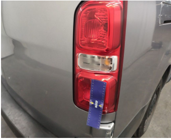
Light / Rear Right / Replace-cracked
