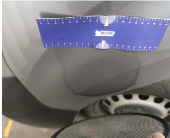
Wing Front Left // Repair & Painting-dent
