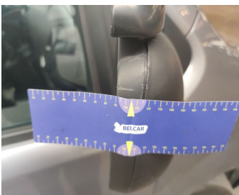
Side View Mirror Right // Replace Not Painted-scratch
