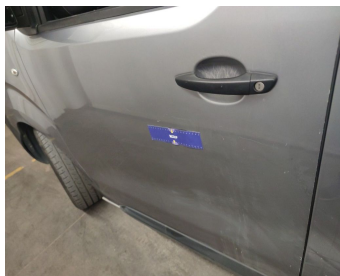
Wing Rear Left / Trim / Replace-scratch
