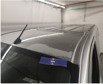
Roof // Painting-Chipped paint
