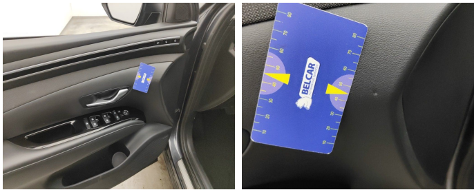
Front Left Door Interior Coating // Replace Completely-hole
