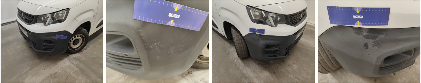
Bumper Front / Lower Cover Not Painted / Replace-stain
