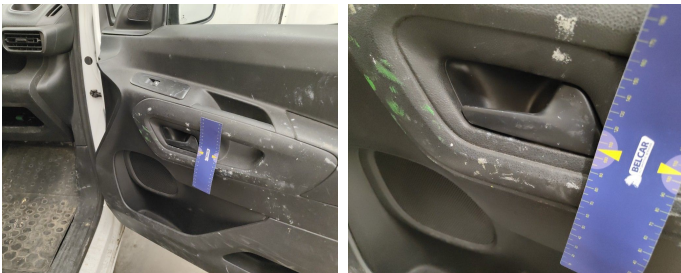
Front Right Door Interior Coating / Door Handle / Replace-stain
