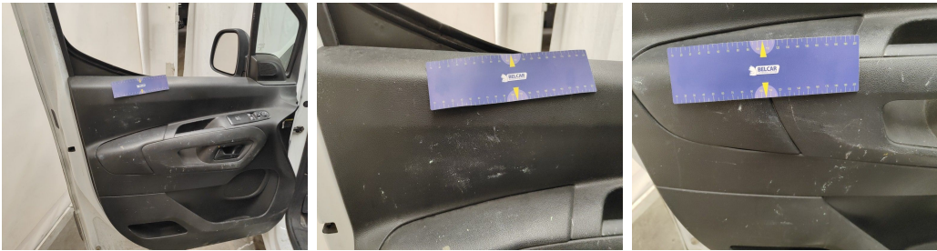
Front Left Door Interior Coating // Replace Completely-stain
