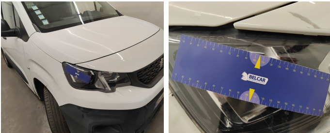
Light / Front Right / Replace-scratch
