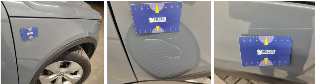
Wing Front right // Repair & Painting-scratch + dent
