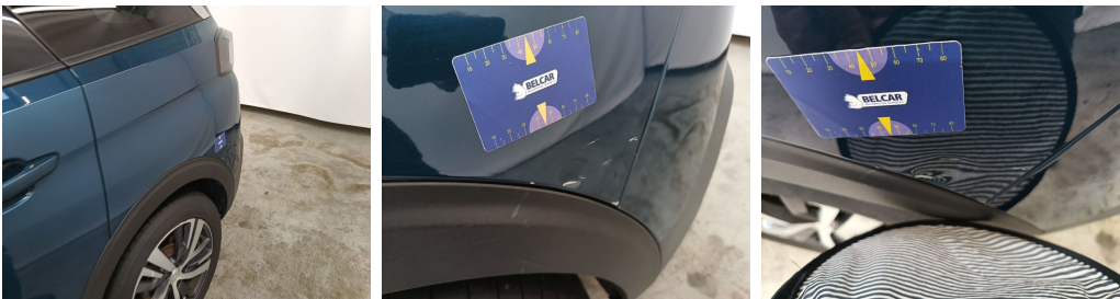
Wing Rear Left // Smart Repair Medium-scratch + dent
