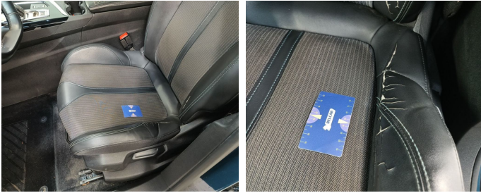
Seat Front Left / Bottom Coating / Replace-worn
