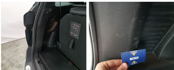
Trunk Compartment / Side Cover Left / Replace-scratch
