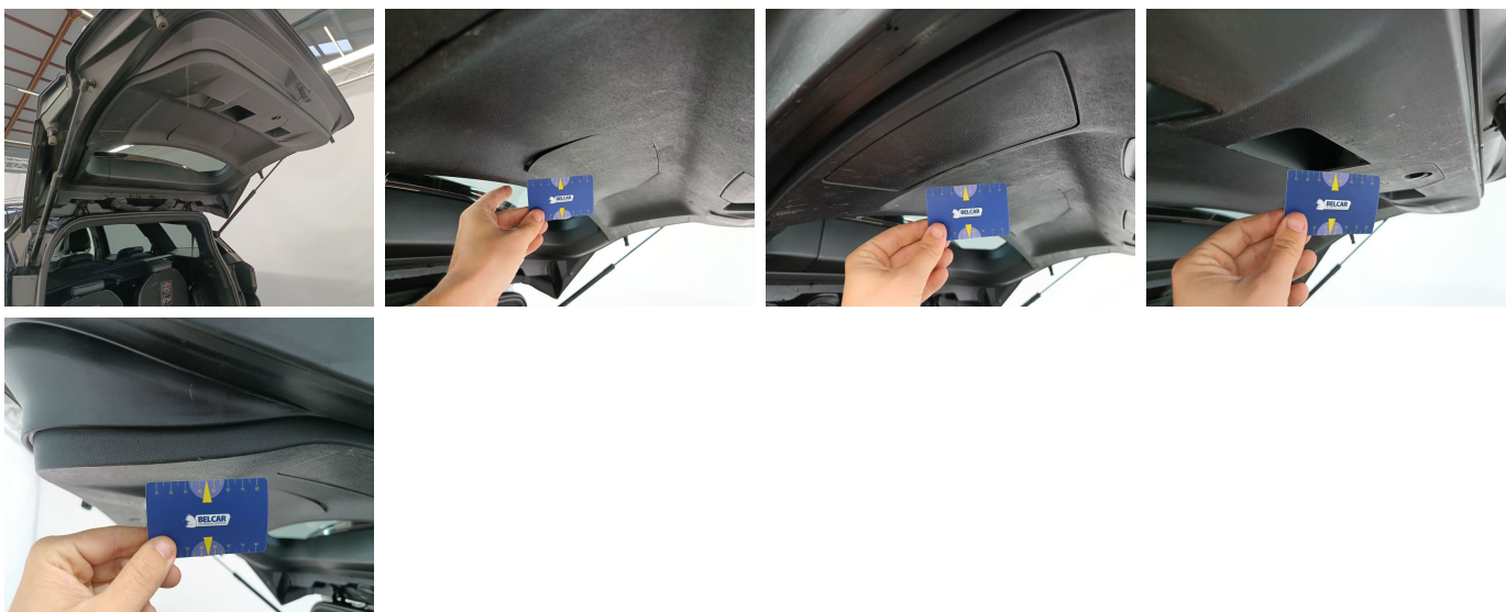
Trunk Lid Interior Coating / Complete Panel / Replace-scratch
