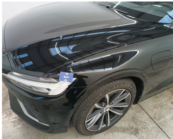
Wing Front Left // Polish-scratch
