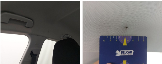
Interior // Repair 2-Incinerated
