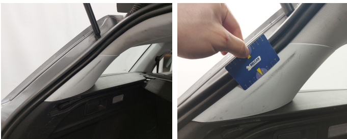
Trunk Compartment / Side Cover Left / Replace-scratch
