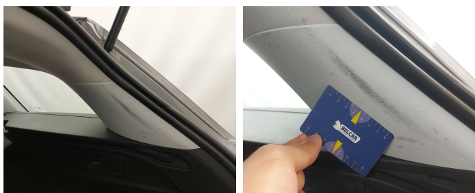
Trunk Compartment / Side Cover Right / Replace-scratch
