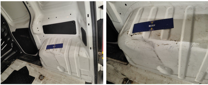
Trunk Compartment / Side Cover Right / Replace-scratch + dent
