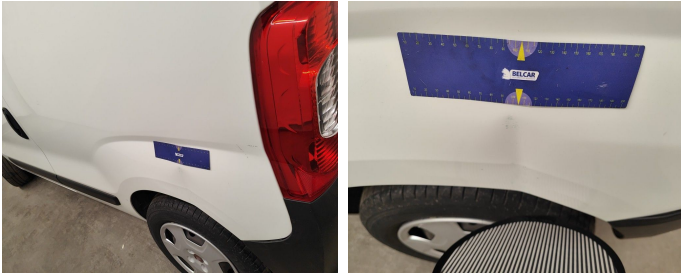
Wing Rear Left // Repair & Painting-dent
