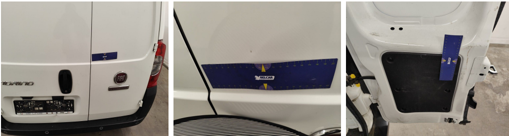
Rear Loading Door Right // Repair & Painting-scratch + dent
