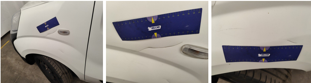
Wing Front Left // Repair & Painting-scratch + dent
