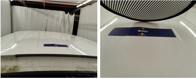
Roof // Smart Repair Medium-dent
