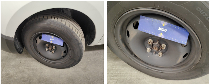
Wheel Front Left / Wheel Cover / Replace-missing
