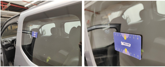
Door Rear Left / Window / Replace-scratch
