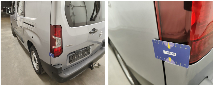
Light / Rear left / Replace-scratch
