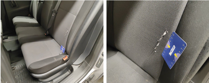
Seat Rear Left / Rear Coating / Replace-worn
