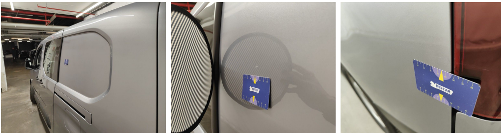
Wing Rear Left // Repair & Painting-scratch + dent
