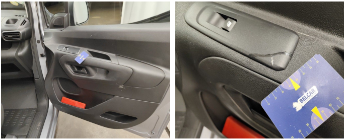
Front Right Door Interior Coating / Control Module / Replace-cracked
