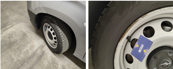
Wheel Steel Front Left // Replace-dent
