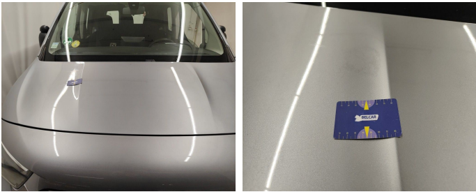
Front Bonnet // Polish-Chemical reaction
