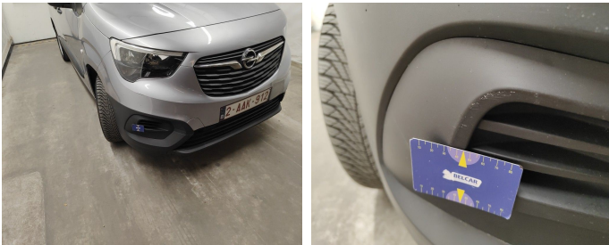
Bumper Front / Grid Right / Replace-scratch
