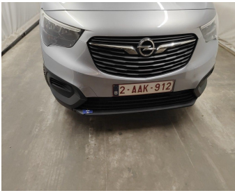
Bumper Front / Lower Cover Not Painted / Replace-scratch
