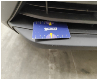
Bumper Front / Lower Cover Not Painted / Replace-scratch
