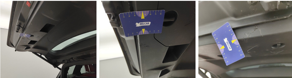
Trunk Lid Interior Coating / Complete Panel / Replace-scratch
