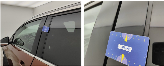
Door Rear Left / Trim / Replace-scratch
