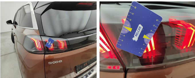
Light / Rear Left On Rear Bonnet / Replace-scratch
