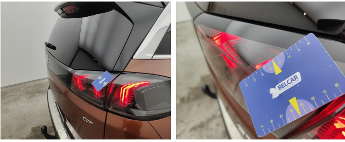
Light / Rear Right On Rear Bonnet / Replace-scratch
