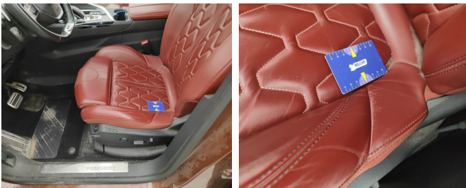
Seat Front Left / Bottom Coating / Replace-worn
