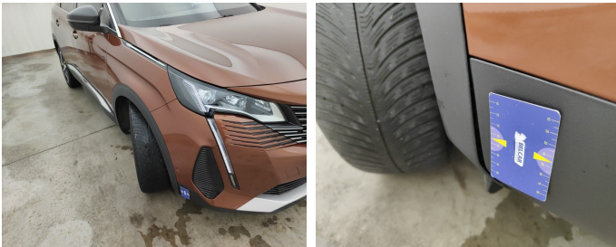
Wing Front right / Trim / Replace-bad position
