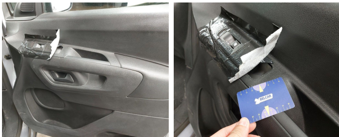
Front Right Door Interior Coating // Replace Completely-cracked
