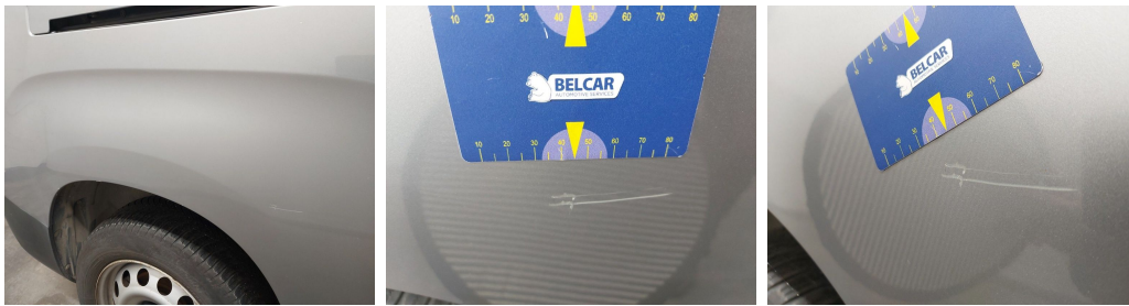
Wing Rear Right // Repair & Painting-scratch + dent
