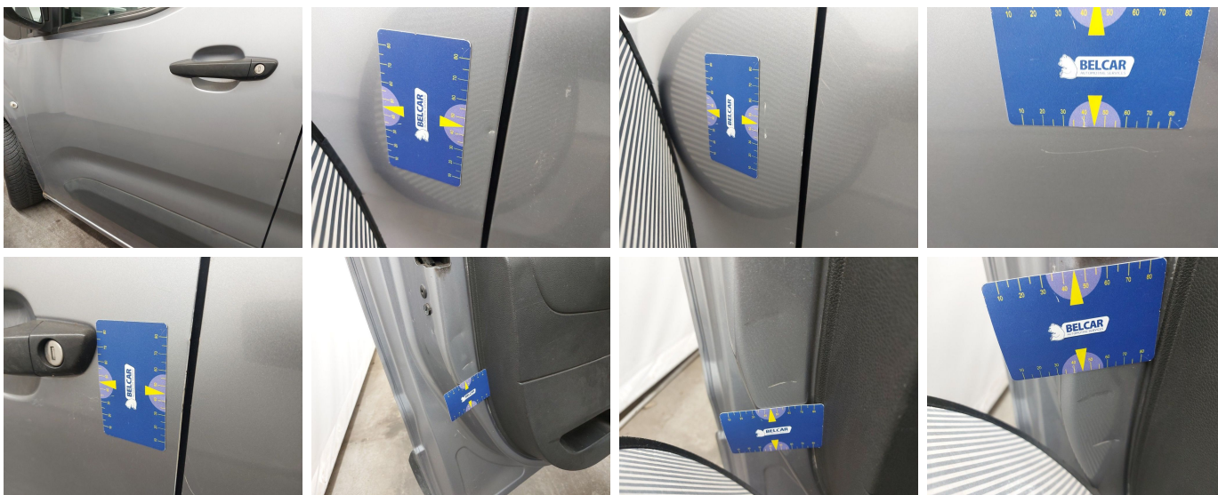
Door Front Left // Repair & Painting-scratch + dent
