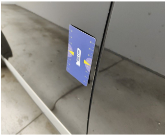
Door Front Left // Repair & Painting-scratch + dent
