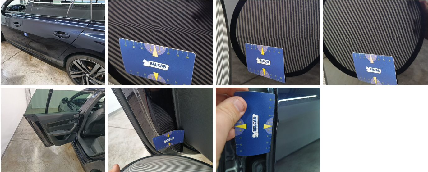
Door Rear Left // Repair & Painting-dent
