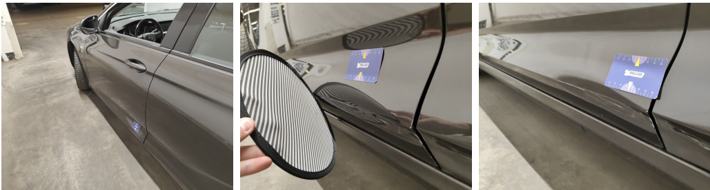
Door Front Left // Repair & Painting-scratch + dent
