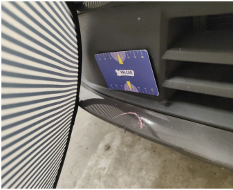
Bumper Front // Repair & Painting-scratch + dent
