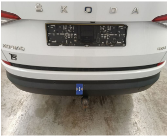
Bumper Rear / Lower Cover Not Painted / Replace-scratch
