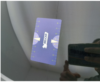
Rear Bonnet / Rear Window / Replace-scratch
