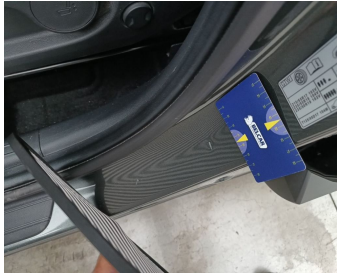
Rocker Panel Left // Smart Repair Medium-scratch + dent
