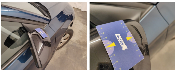
Side View Mirror Right / Shell / Replace Painted-cracked
