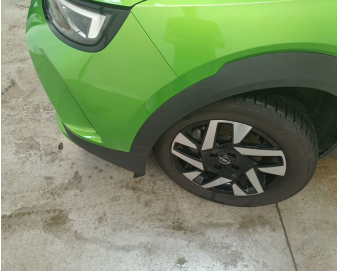
Wing Front Left / Trim / Replace-scratch
