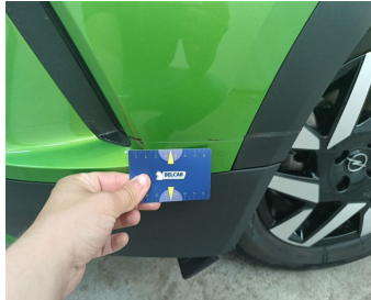
Wing Front Left / Trim / Replace-scratch
