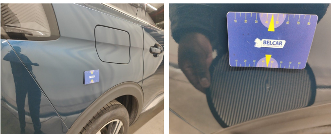
Wing Rear Right // Repair & Painting-scratch + dent
