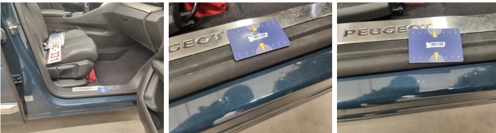
Rocker Panel Right // Smart Repair Medium-scratch + dent
