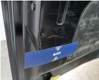
Rear Loading Door Left // Repair & Painting-scratch + dent
