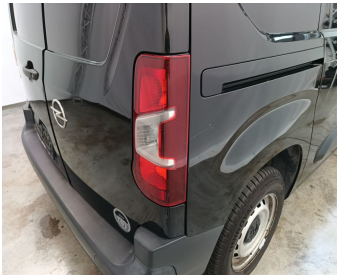
Light / Rear Right / Replace-scratch
