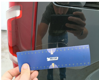
Door Rear Right // Repair & Painting-scratch
