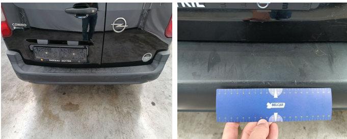
Bumper Rear // Replace without painting-scratch
