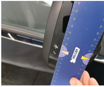
Side View Mirror Right // Painting-scratch
