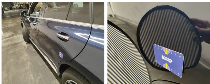
Door Rear Left // Painting-bad repair
