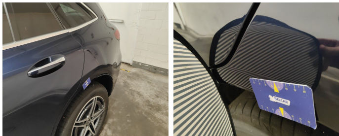
Wing Rear Left // Painting-bad repair
