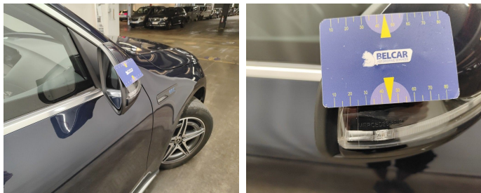
Side View Mirror Right / Direction Indicator / Replace-scratch
