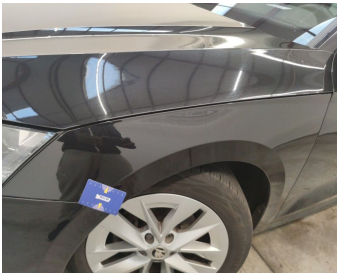
Wing Front Left // Painting-bad repair
