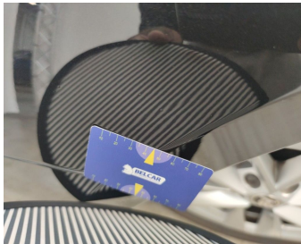
Wing Front Left // Painting-bad repair
