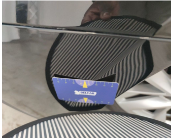
Rocker Panel Left // Smart Repair Medium-scratch + dent
