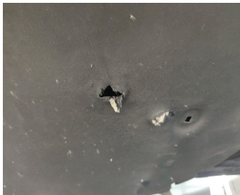
Front Bonnet / Insulation / Replace-cracked
