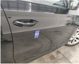
Door Front Right // Painting-scratch
