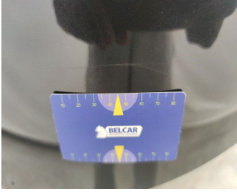
Bumper Rear // Painting-scratch
