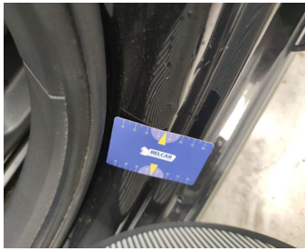
Rocker Panel Left // Smart Repair Medium-scratch + dent
