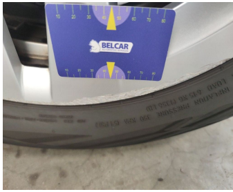
Wheel Alloy Front Right // Repair-scratch
