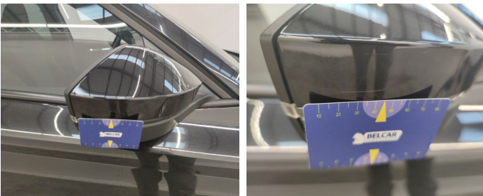
Side View Mirror Right // Painting-scratch
