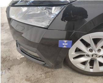
Bumper Front // Painting-bad repair
