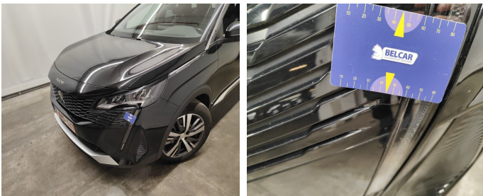
Bumper Front / Trim Left / Replace-scratch
