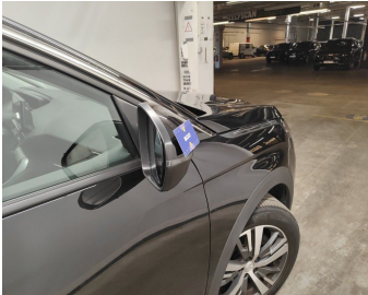
Side View Mirror Right / Direction Indicator / Replace-scratch
