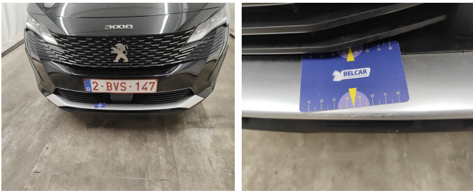
Bumper Front / Spoiler / Replace-scratch
