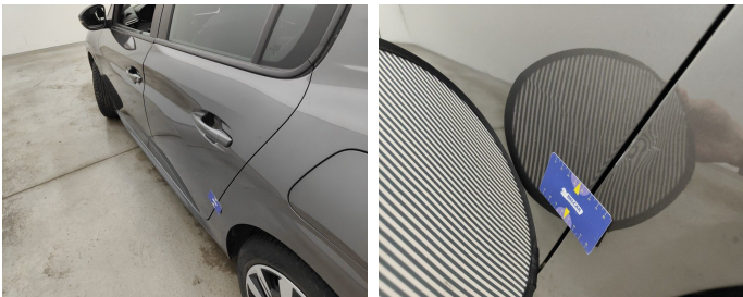
Door Rear Left // Repair & Painting-scratch + dent
