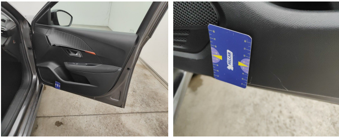
Front Right Door Interior Coating // Replace Completely-scratch
