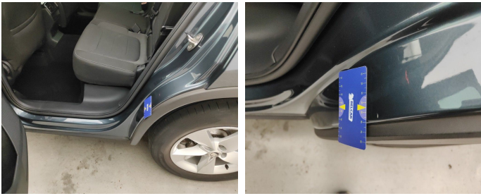
Rocker Panel Left // Smart Repair Medium-scratch
