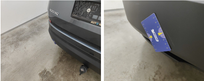
Bumper Rear / Lower Cover Not Painted / Replace-scratch
