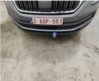
Bumper Front / Lower Cover Not Painted / Replace-scratch
